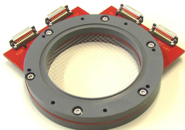
Fig. 2 – Photograph of the applied wire-mesh sensor.
