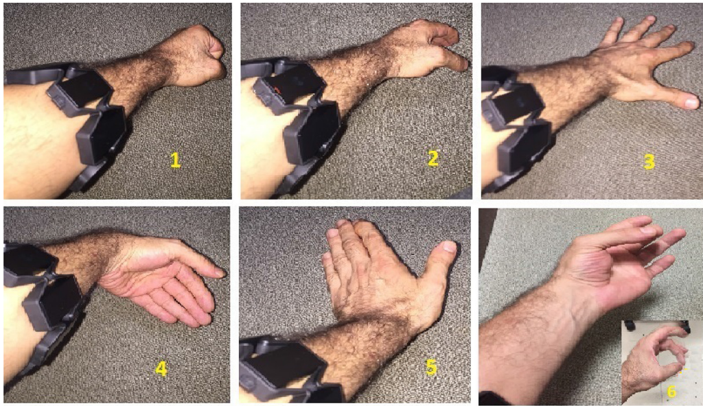
Fig. 2. MYO hand gestures, 1 – fist, 2 – hand relax, 3 – finger spread, 4 – wave in, 5 – wave out, 6 – double tap.
