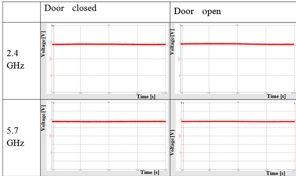
Fig. 10 – Output data of the plant control system (PCS) cabinet for immunity evaluation.
