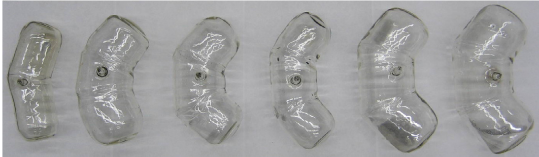
Fig. 2. Six wide angle cells denoted by “Veronica”, “Archie”, “Reggie”, “Jughead”, “Reliance” and “Giant”, from left to right. The cell Veronica was the first test of the fabrication method and is made from only two sections of GE180 glass, whereas the other cells are made from three sections.
