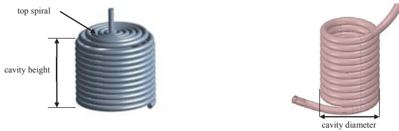
Fig. 2 Receiving cavity optimization parameters: with top spiral (l.h.s.) without top spiral (r.h.s.)
