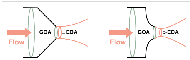
Figure 2. Effect of Valve Shape on EOA
