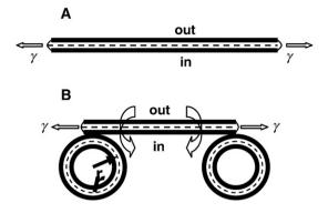
**Fig. A1.** Illustration of the model. A.) Initial state: flat bilayer subjected to lateral tension. B.) Vesiculated state: formed vesicles and the remaining flat bilayer. The bent arrows show the direction of lipid transfer by flippases.
