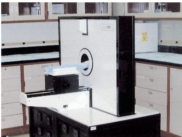
Figure 2. MicroPET scanner developed at UCLA for high-resolution PET imaging of small animals. Shown is the first-generation microPET scanner. The scanner has a transverse field of view of 11 cm and an axial field of view of 1.8 cm. The spatial resolution of the scanner is \sim 1.8^3 \text{ mm}^3 . An entire mouse can be scanned using multiple bed positions in 30 to 60 minutes. Newer versions of this scanner will allow for \sim 1^3 \text{ mm}^3 spatial resolution and scanning times for an entire mouse in under 10 minutes.
