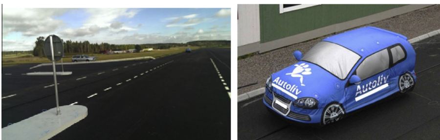
Fig. 4. The test-track intersection (left), and the balloon car used in the study (right).
