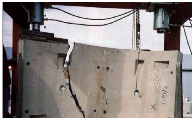
Fig. 4: Example of fibre-reinforced concrete tubing element examined in the natural scale [6]
