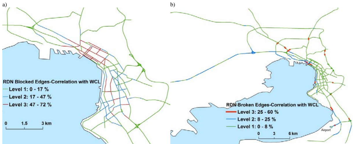
Fig. 2. Correlation of a) blocked by buildings edges and b) broken edges (damaged bridges and road segments) to road network connectivity.
