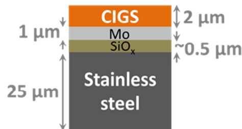
Fig. 1. Sketch of the sample cross section used for the scribing experiments.
