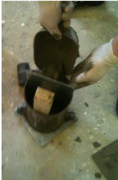
Fig. 3. Pouring the non-monolithic cylinders.
