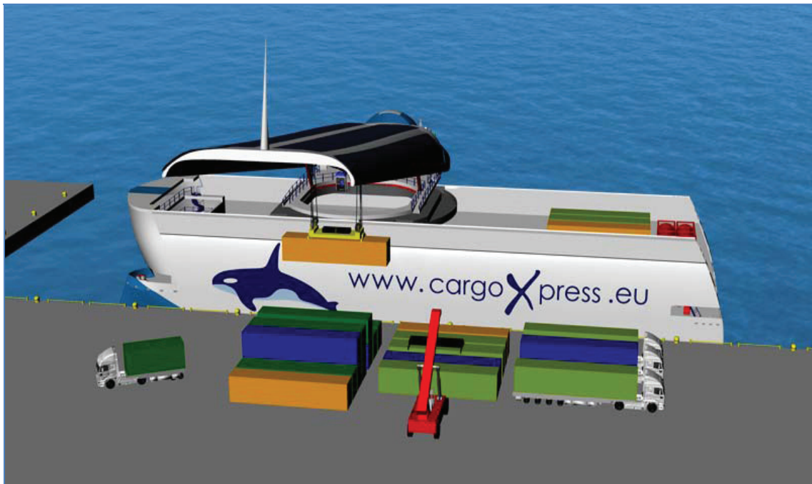
Fig.1: 3D overview of new cargo-vessel with cantilevering on-board crane. Source Innovacion Logistica SL (ILCX)
