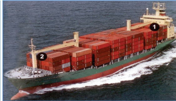
Fig.2b: Feeder vessel with on-board jib-cranes source: Dokmar Maritime Publishers B.V. 6 th Edition.
