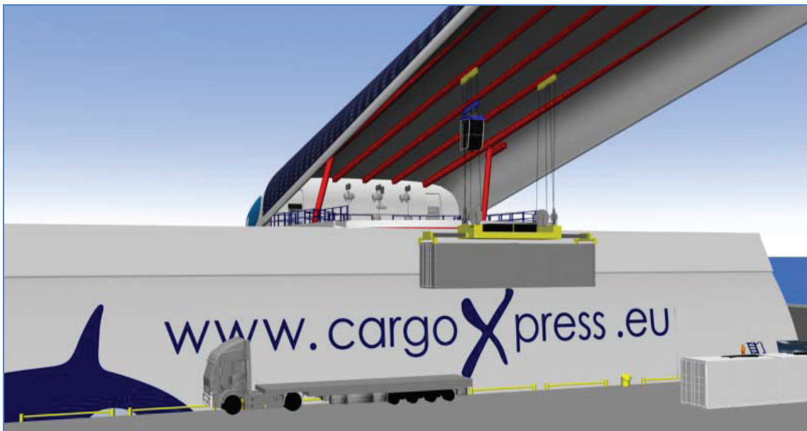
Fig. 10: View from quay to crane unloading a 40-foot container, the control cabin hanging in the middle rail. Source: ILCX
