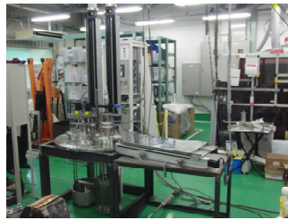
Fig. 12 New electrorefiner with high-temperature fluid transport system.
