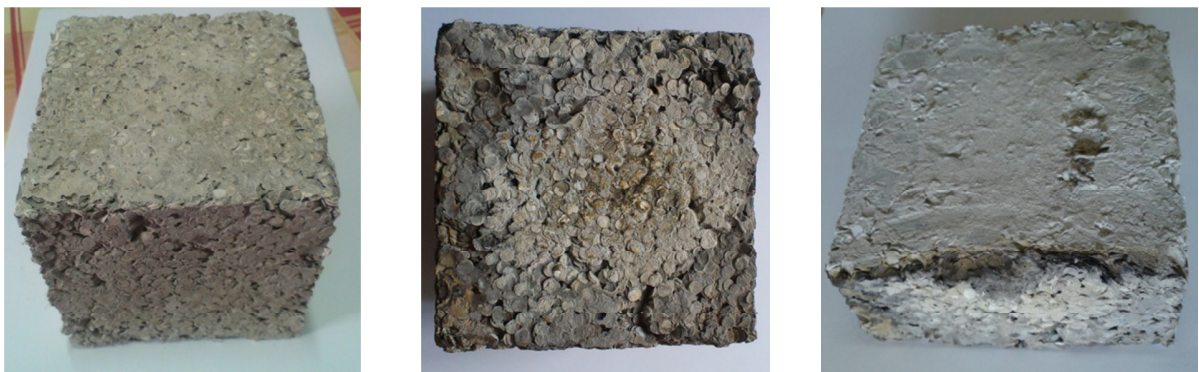
a) Copy paper mortar test tube b) Test tube burned with the gas lamp for 5 minutes c) Cross-section of the burned test tube
