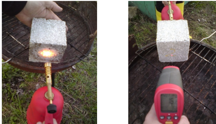
a) Copy paper test tube burned with the gas lamp b) Temperature recorded in the side opposite to fire exposure
