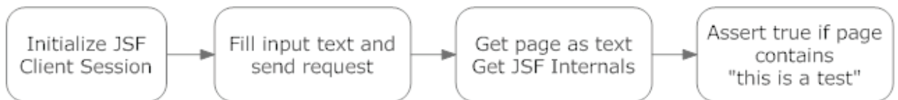
Figure 4. JSFUnit automatic test steps
