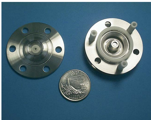
Figure 1. Photograph of the miniature toroidal rf ion trap analyzer showing the filament endcap (left) removed to expose the ion storage region (right). A U.S. quarter-dollar coin provides a size perspective.
