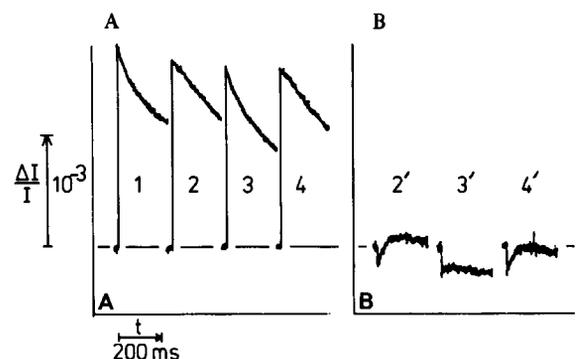
Fig.4. Transmembrane electrical field increase (upward) and decrease, recorded as electrochromic absorbance changes, during the first 220 ms after each of 4 flashes spaced by 1.2 s intervals. Average of 16 pairs of measurements (515 nm minus 500 nm). Dark time before the measurements, 4–5.5 h. Chlorophyll, 60  $\mu$ g/ml. Curves 2'–4' represent the difference between curves 2–4 and curve 1.
