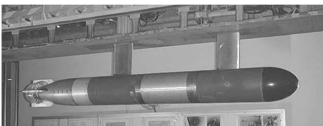
Fig. 4 Model and PJP assembly on test section.
