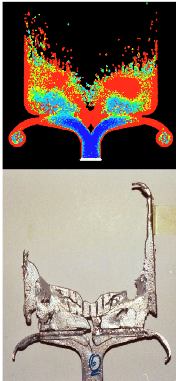
Fig. 6. Short shot with 25% volume fill: simulation (top) with colour representing viscosity, blue being low and red high; and experiment (bottom). For T_{DIE} = 27 °C and liquid metal super-heat T_{AL} = 0 °C. (For interpretation of the references to colour in this figure legend, the reader is referred to the web version of this article.)
