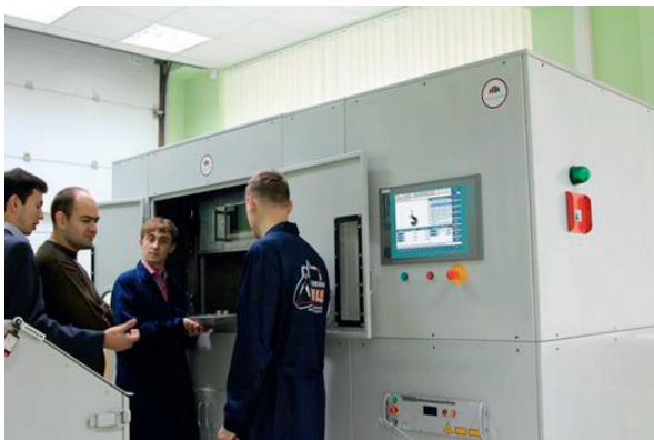
Fig. 5. Selective laser sintering machine with control system.
