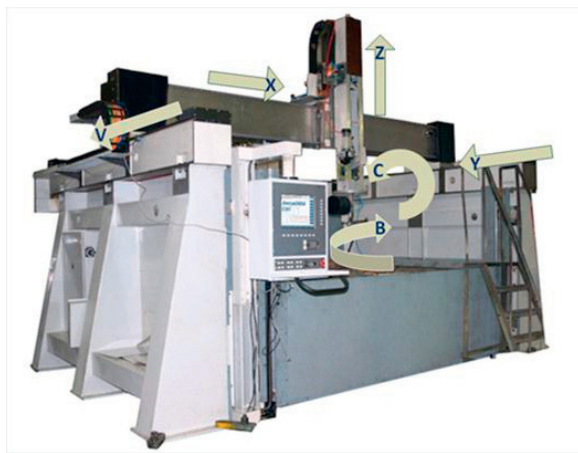
Fig. 8. The water jet cutting machine tool.
