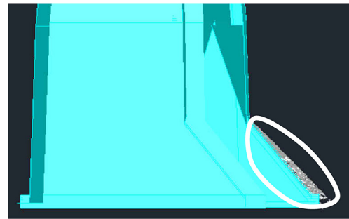
Figure 16 As built model has wider base from the design model.
