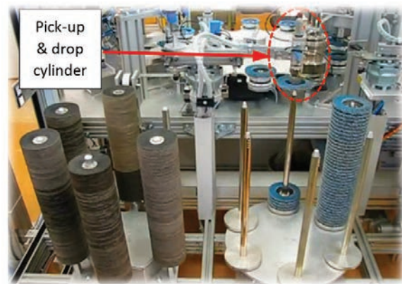
Fig. 4. Flap discs manufacturing machine.
