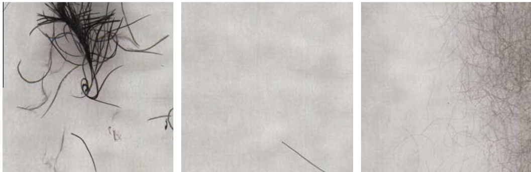
Fig. 3 – Acquired color image examples: (a) opened chicken feather, (b) opened hair, and (c) opened black fiber cloth.
