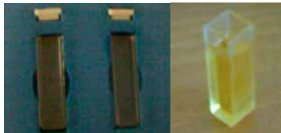
Fig. 1. Cuvette holder and cuvette containing oil sample
