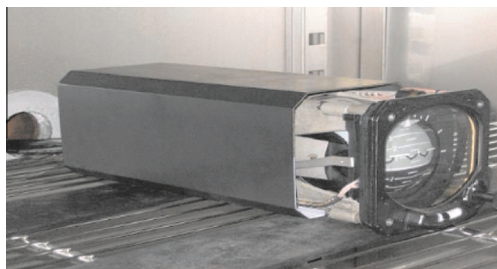
Fig. 6 Environmental test of the gyroscope.
