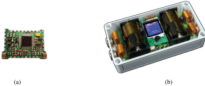
Fig. 3. (a) implemented measurement module (SMT) with a dimension of 30 mm (W) - 20 mm (D) - 4.2 mm (H), and (b) the outdoor device with four SMT modules
