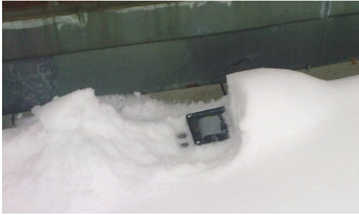
Fig. 4. Long term test of the developed instrument, under harsh conditions with over 10 cm of snow.
