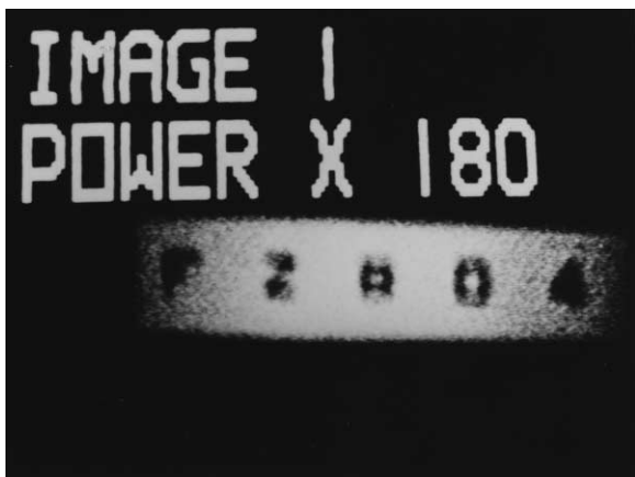
Fig. 1. Illustration from the literature showing blur produced by a \pm eighth diopter cross cylinder placed in front of a camera. It is clear that the optical effects are grossly exaggerated and do not simulate the blur of out-of-focus ocular imagery (From Sims CN & Durham DG, 1986. The Jackson cross-cylinder disproved. Transactions of the American Ophthalmological Society , 86, 355–386. Photograph reproduced with permission of the American Ophthalmological Society).
