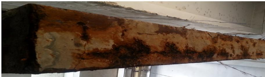
Fig. 11 The deterioration of the concrete against corroded rebar for samples.
