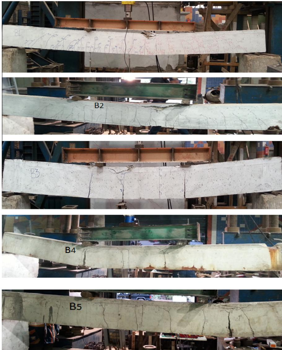
Fig. 10 Crack pattern and failure for specimens.
