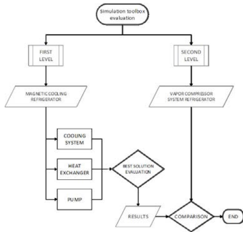
Fig. 3. Logic description of Decision Support Toolbox algorithm applied to refrigeration system.
