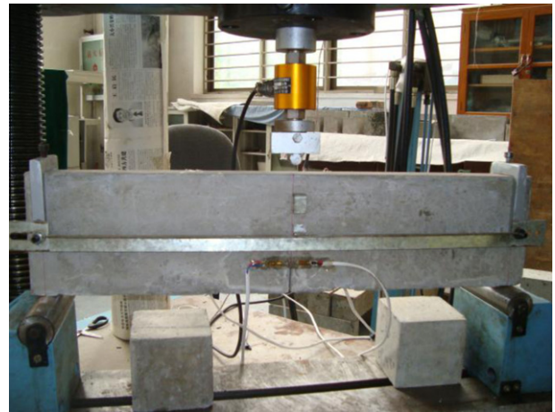
Fig. 4. Set-up of the three-point bending beam test.
