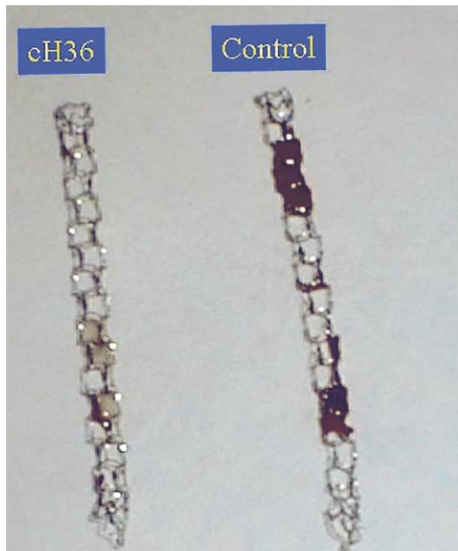
Figure 1. Thrombus formation after 120 min perfusion on stent surface exposed to blood pretreated with either saline (control) or with a monoclonal antibody against tissue factor (cH36). Note the striking reduction of thrombus formation on the stent in which blood was pretreated with cH36.
