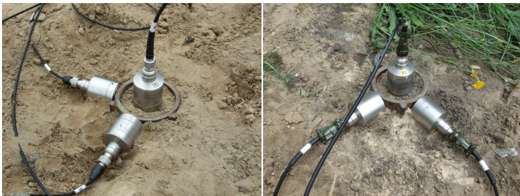
Figure 2: A view of measurement points (MP1 and MP2) with attached seismic sensors
