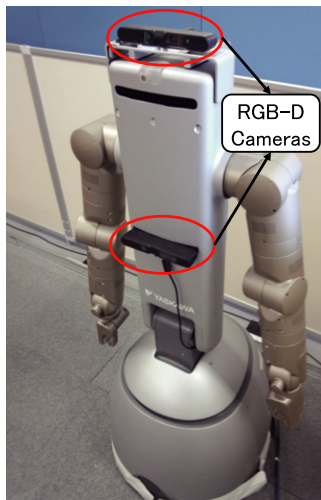
Fig. 8. SmartPal-V is equipped with two RGB-D cameras.
