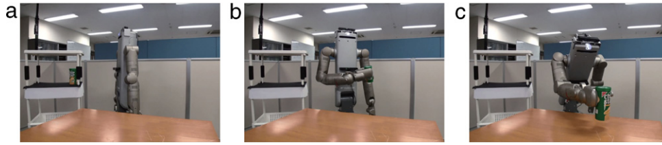
Fig. 24. Goods gripping experiment: (a) initial state, (b) intermediate position, (c) goods delivery attitude.
