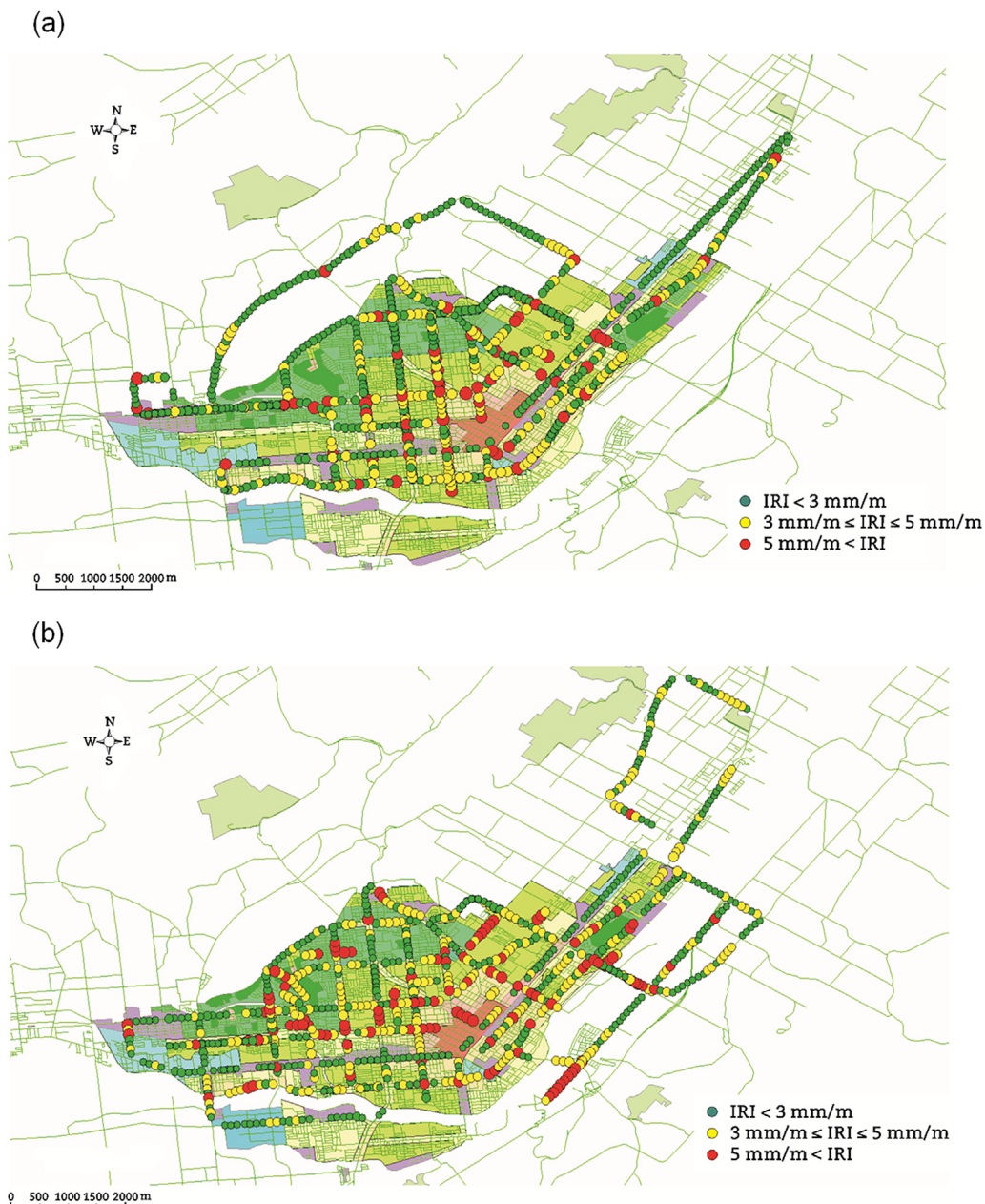
Fig. 6 – IRI based on the digital road map and GIS examples of city A. (a) In 2011. (b) In 2013.
