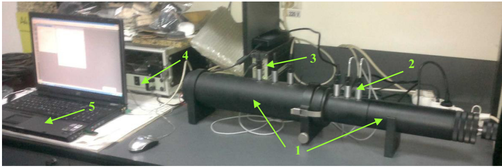
Fig. 4. Experimental stand used for the sound absorption coefficient measurement
