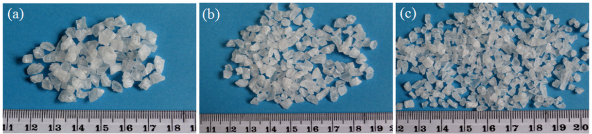
Fig. 2. Digital images showing the NaCl particles sizes used in the processing of the aluminum foams: a) NaCl particle size from 4.7 to 4.0 mm (range I), b) NaCl particle size from 4.0 to 3.3 mm (range II), and c) NaCl particle size from 3.3 to 2.0 mm (range III).
