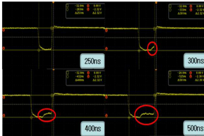
Fig. 4. Pulse Shape with the Different Pulse Widths
