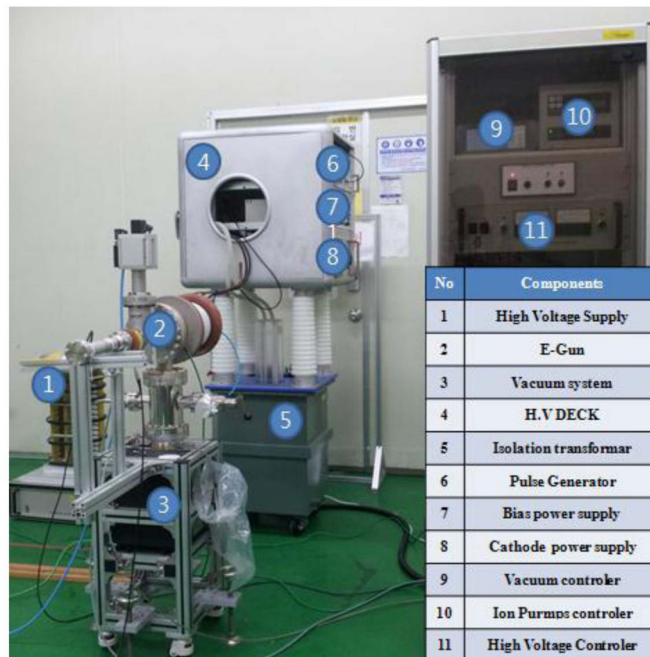
Fig. 3. Actual Appearance of the Electron Generator System
