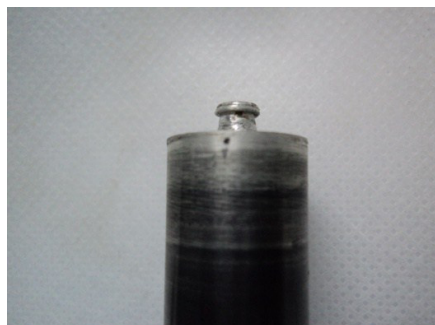
Fig.4. Shape of tool pin after welding
