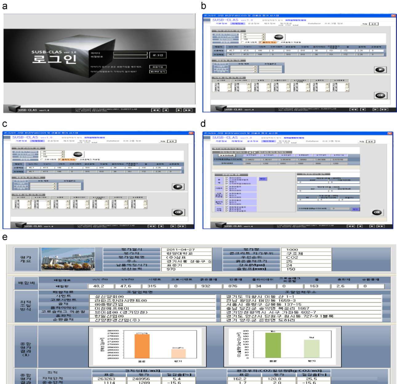
Fig. 7. Optimal design system for CO 2 emissions and cost in the life cycle of concrete. (a) Program main screen, (b) Basic Information Input Sheet, (c) Materials Stage Input Sheet, (d) Production Stage Input Sheet and (e) Evaluation Results Sheet.
