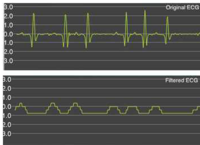
Fig. 5. The QRS detection algorithm processing result
