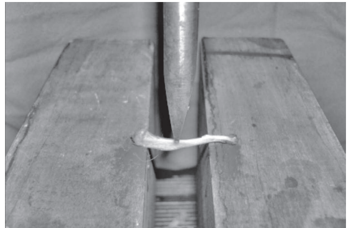
Figure 2 – Detail of the specimen at rest and the load application blade positioned halfway between the ends.
