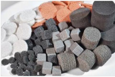
Fig. 8. The Alantum foam pellets used in applications to chemical processes
