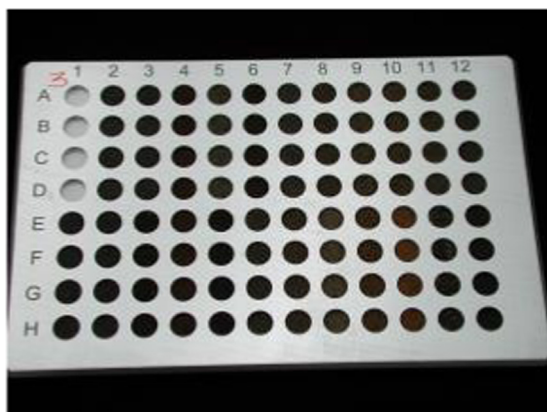
Fig. 4. Aluminum plate with sample-filled micro-titer engraved wells.
