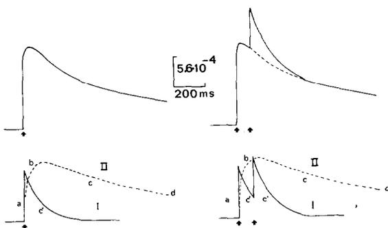
Fig.2. Resolution (bottom part of the figure), of the  $\Delta A$  induced by a single and a double flash into two components; reaction I (solid curve) and reaction II (broken curve). Curves I and II were computed according to the data obtained from the curve analysis depicted in fig.1. Further explanations are in the text.
