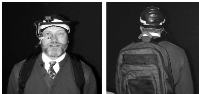
Fig. 2. Recording apparatus mounted on a person. Images of eye and scene were recorded with an ISCAN headband-mounted, eye and line-of-sight scene video-based imaging system. The system was modified to be battery operated. The cameras outputs were recorded on synchronized, digital video camcorders carried in a backpack and analyzed offline.
