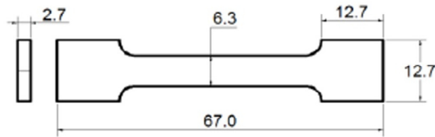
Fig. 2. Injection mold part and geometry. Dimensions are in mm.
