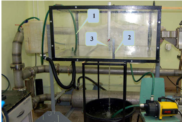
Fig. 1. Experimental tank. 1 – the water supply tube, 2 – a ruler, 3 – the separator is placing above the drain hole.
