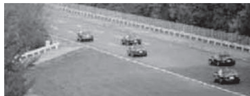
Fig. 8 Cooperative driving with 5 automated vehicles linked by inter-vehicle communications in 2000
