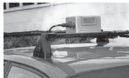
Fig. 4 Inter-vehicle communication unit developed during PROMETHEUS project in 1994
